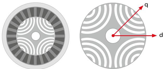
The torque produced by a synchronous reluctance motor is proportional to the difference between the inductances on the d- and q-axes: the greater this difference, the greater the torque production. Synchronous reluctance motors are therefore designed with magnetically conductive material, iron, in the d-axis and magnetically insulating material, air, in the q-axis.
